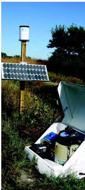
For the many customers who already use Flowlink Pro, remote sampler communication and water quality data retrieval can easily be integrated into an established monitoring system.
