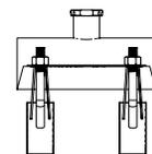
Each saddle has a range of actual pipe size O.D. that it will work with. When you order your meter, you will specify the nominal pipe size and the saddle provided will work with the following actual pipe O.D.
