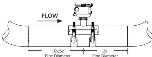
Upstream straight pipe is selected during initial setup. Upstream options are 5X or 10X the diameter and are based on the amount of straight pipe available in either new or propeller meter replacement installation. Downstream straight pipe requirement is 2X the diameter. See programming setup for details.
